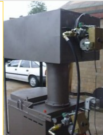
DEFRA approved incinerator with the secondary chamber
