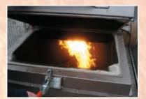
One of the main features of our incinerator range is that they burn virtually smoke and smell free without the need for a secondary burner because of their patented internal design. Their simplicity of operation make the units a key benefit on any waste disposal application by avoiding the need for constant supervision.
