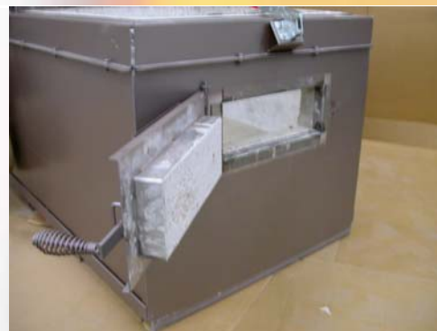
Front ash removal door
